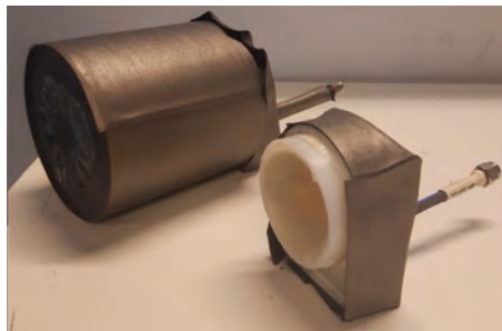
Figure 1. Dielectric Rod Antenna (left) and Self Grounded Bow-Tie Antenna (right)
